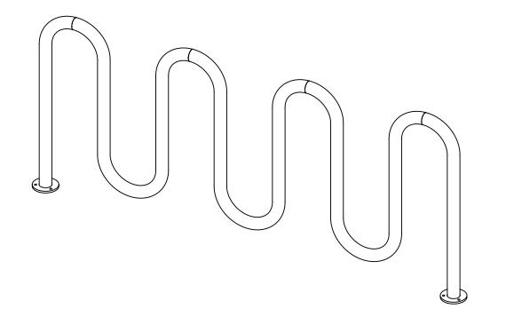
The English Walnut Bike Rack is constructed of continuous cold rolled steel. The bike rack is fully welded with no overlapping surfaces where moisture can be trapped. The bench is sandblasted to a SSPC-SP 5/NACE standard "white finish", epoxy primed, and powder coated with a "Super Durable TGIC" polyester top coat in the color of your choice.
